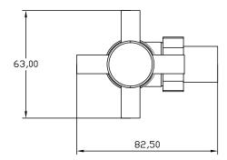
Please note due to manufacturing tolerances pipe centres may vary by +/- 10mm, we recommend that pipe work is not altered until your towel rail / radiator is on site. The information contained on this page was correct at date of issue. Fitting dimensions are provided as a guide only. We pursue a policy of continuing improvement in design and performance of our products and so reserve the right to change specifications without prior notice.
